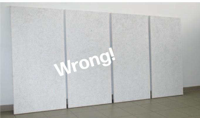
Never lean the acoustic panels on an angle against the wall during installation and subsequent painting. This causes the panels to warp - warped panels can no longer be installed.
