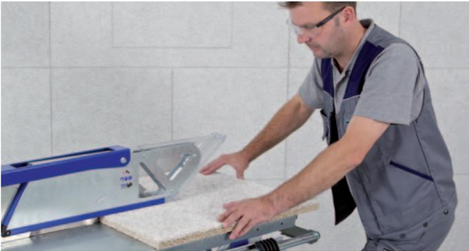
**Table saw** - Lay the acoustic panel down with the exposed side up. Always work with a safety guard, guide and an extraction system.
