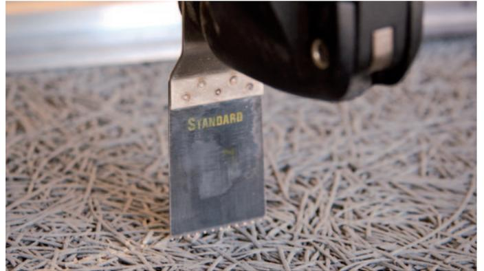
**Cutting openings by means of a supercutter** - Only cut at a right angle to the panel surface.
