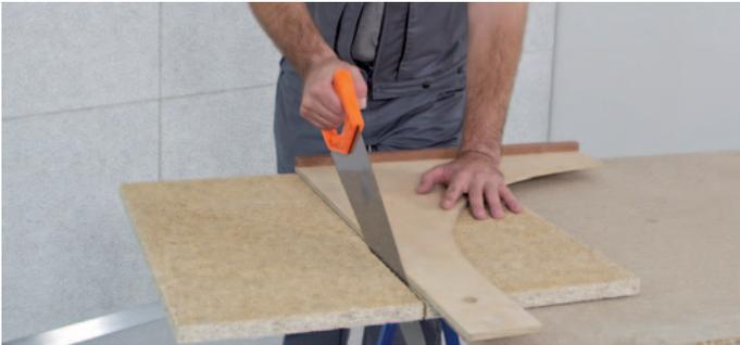
**Jack saw** - Lay the acoustic panel down with the exposed side up. Always work with a guide. Support the free end of the panel.
