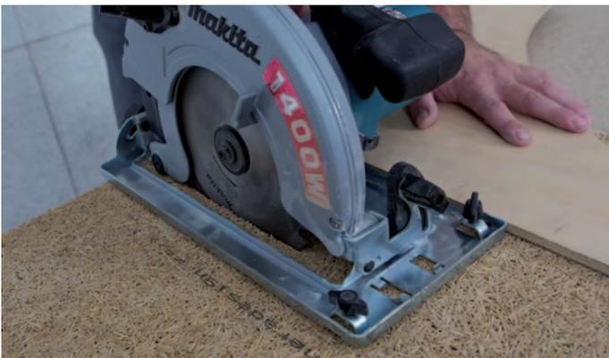
**Circular saw** - Lay the acoustic panel down with the exposed side down. Always work with a guide and an extraction system. Support the free end of the panel.
