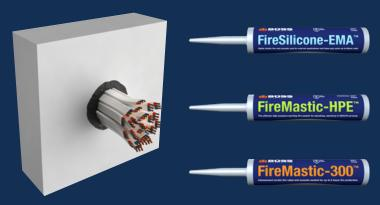
**FireSilicone-EMA™** is a fire resistant silicone sealant. It is a one-part, neutral curing silicone for construction joints and service penetrations. With excellent flexibility and weatherability, it offers up to 300 minutes fire resistance. It can also be used to seal a variety of power and communications cables in walls and floors when partnered with BOSS Thermal Defence Wrap.
