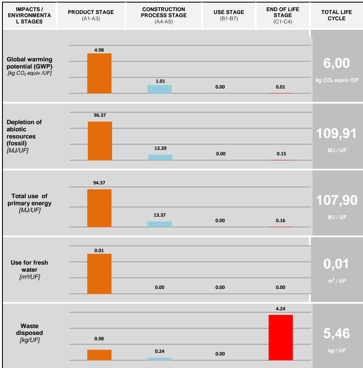
Figure 6-1: Relative contributions of different life cycle processes to the environmental effects and primary energy utilisation of 1m 2 of mineral board (19mm) 230kg/m 3 density
