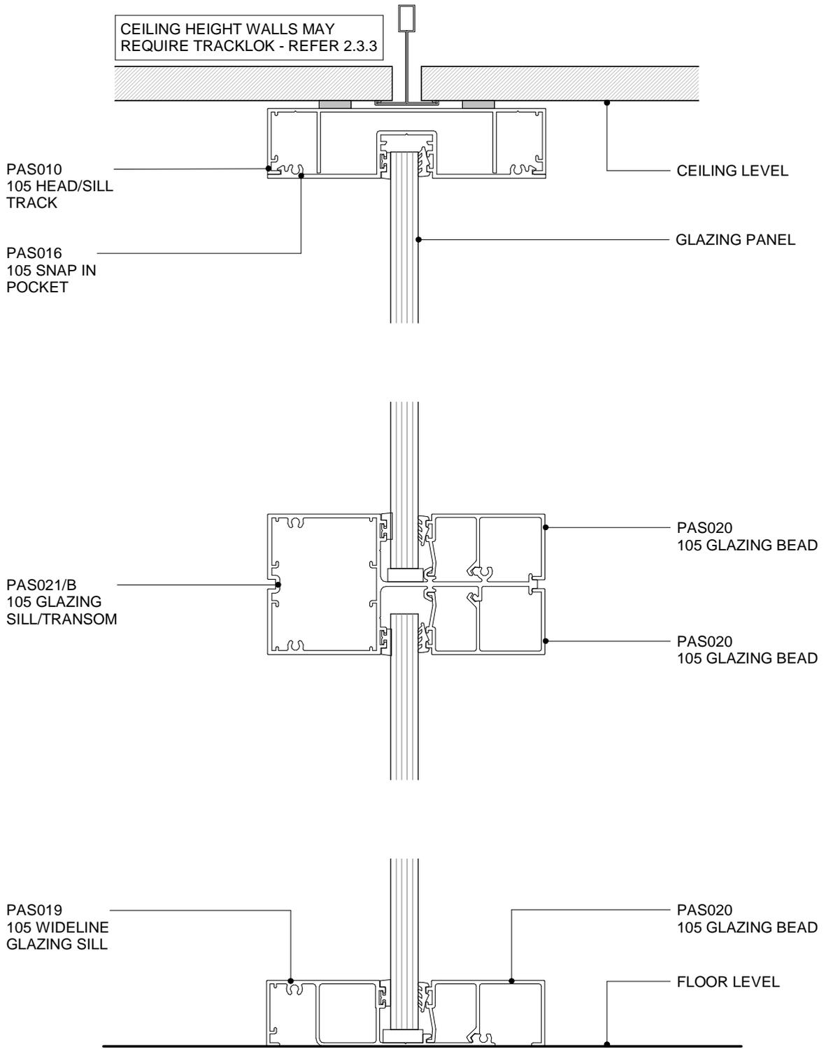
**TRANSOM MAX SPAN IS 1200MM. FOR LARGER SPANS, CONTACT POTTERS SPEC TEAM**
