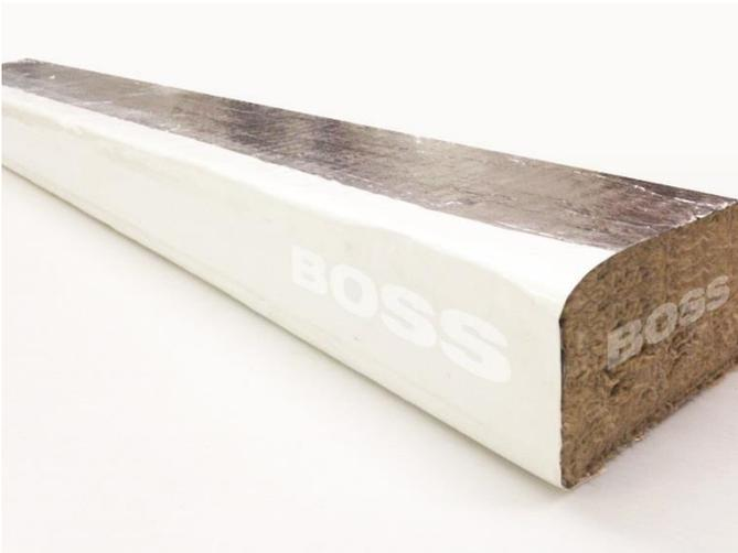
Rainscreen Ventilated Fire Barrier (RSVB) is developed to protect the building void between the outer rainscreen cladding/facade and the inner construction element. **RSVB** leaves a gap up to 50mm to allow the movement of air and moisture. The aluminium foil facings provide class 'O' rating and excellent resistance to smoke. A unique method of manufacture provides a resilient lateral compression required to ensure a tight fit.
