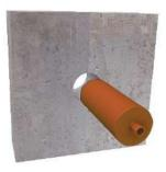
Ensure the opening and any surface / substrate which the product will come into contact with is clean, dry, free of dust and loose particles and free from oil or grease.
