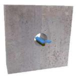
4. Mask the surface of the wall if an aesthetic finish is required. Install the service and pack the aperture if required with foam backing road to control the sealant depth on each side in accordance with the tested or certified system.
