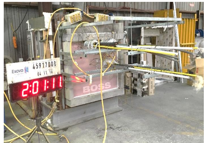
The BOSS FyreBox™ shown on the right during a fire test just after 120 minutes.
