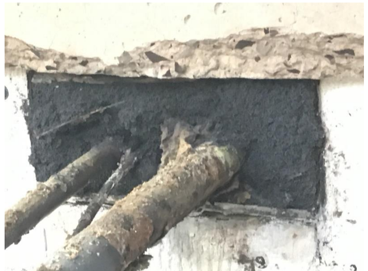
The BOSS FyreBox™ shown on the right during a fire test just after 120 minutes.
