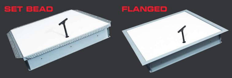
Our Flanged and Set Bead Standard Hatches are available in a range of sizes. The frames are made in New Zealand from strong 0.95BMT Z275 steel with punched folded tab system ensuring strength and square dimensions.
