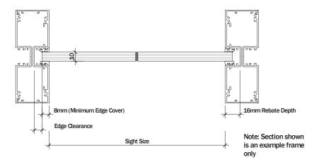
Detail 2. Shuffle Glazing Tolerances
