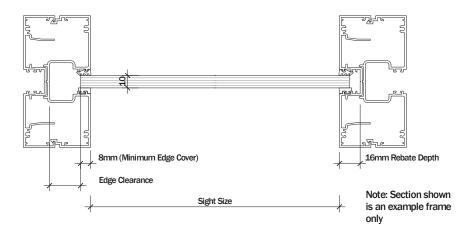
Note. Edge cover is defined as fully supporting the glass – glazing gasket or wedge extending beyond the frame backing should not be considered as part of the edge cover.
