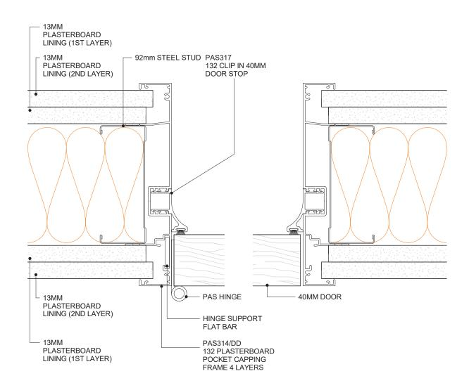
NOTE: DETAIL SIMILAR FOR 3 LAYER FRAME. PAS314/SD POCKET CAPPING FRAME USED IN LIEU OF PAS314/DD
