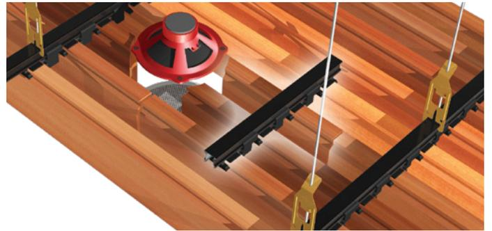
5. Ensure that any smaller joints are properly supported with a short TCR rail and clips covering the adjacent profiles.
