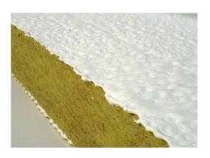
They are a lightweight mineral fibre board that can be easily cut to size on site for simple friction fit applications. Simply push it in to place to fit the aperture and seal the perimeter with FireMastic-300™ fire rated sealant or our specially designed Ablative Coating for bonding Batts to Substrates. For higher insulation performance on services the addition of BOSS products such as P40-MAK Wrap or Thermal Defence Wrap may be used.
