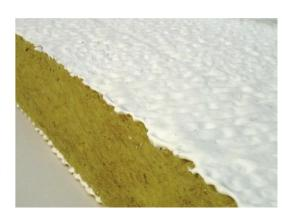
They are a lightweight mineral fibre board that can be easily cut to size on site for simple friction fit applications. Simply push it in to place to fit the aperture and seal the perimeter with FireMastic-300™ fire rated sealant or our specially designed Ablative Coating for bonding Batts to Substrates. For higher insulation performance on services the addition of BOSS products such as P40-MAK Wrap or Thermal Defence Wrap may be used.
