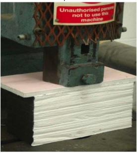
**FlexiCoat-MAK** under 7 tonne load pressure allowing compression to less than 80mm.
