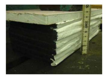
**FlexiCoat-MAK@** 2.5mm WFT cured on elastomeric substrate to perform tests.
