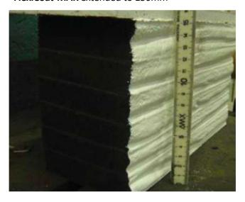
After 1000 cycles there was no visible or physical deterioration of the **FlexiCoat-MAK.**
