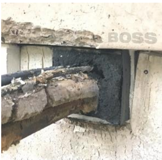
BOSS FyreBox™ 150mm and 300mm shown above after successfully passing a 120minute AS1530.4:2014 Fire Resistance test at Warringtonfire, Dandenong VIC . The images show the intumescent seals inside the BOSS FyreBox™ expand and completely seal around the services passing through the FyreBox™.
