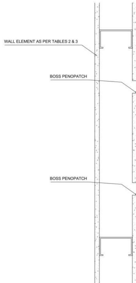
Figure 7 - PEX Pipe or PVC Conduit penetrating the wall without exiting to the other side
