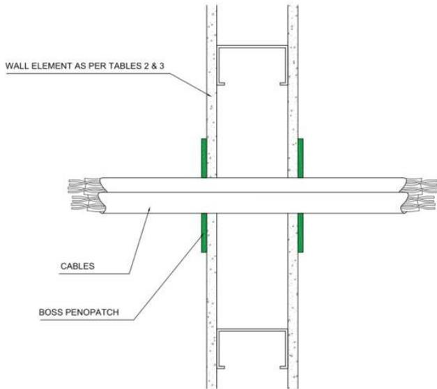
Figure 5 – Cable Penetrations with additional protection
