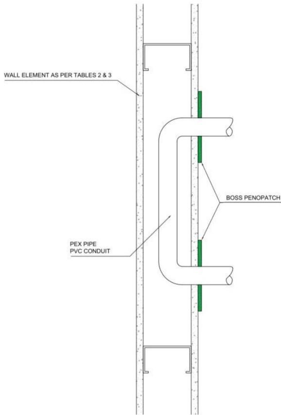
Figure 9 – CAT6 Cable Penetrations (up to 3 cables) penetrating the wall without exiting to the other side
