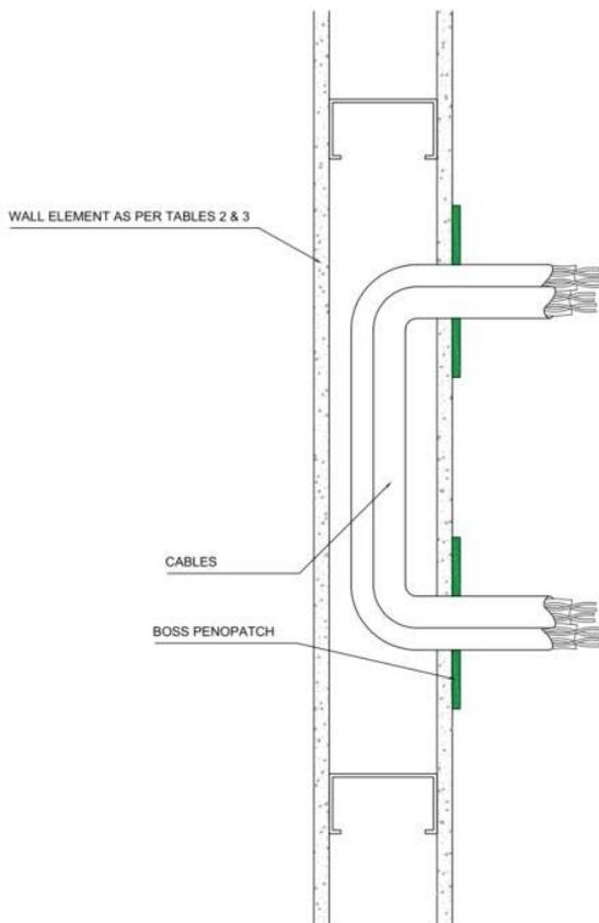
Figure 10 - Cable Penetrations with additional protection penetrating the wall without exiting to the other side
