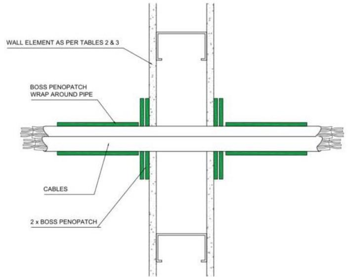
Figure 6 – Blank Seal on the same side of the wall
