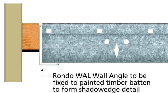
■ LONG LEG WALL ANGLE TYPICAL APPLICATION
