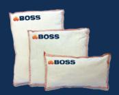
incorporate copper, steel & iron pipes where up to 3 hours integrity and 2 hours insulation are required. BOSS FirePillows-240™ are treated fabric bags containing fire retardant granulated rockwool, securing penetrations in fire rated construction against the spread of fire.
