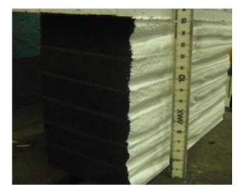
After 1000 cycles there was no visable or physical deterioration of the FlexiCoat-MAK.
