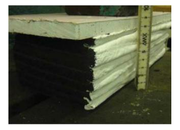
FlexiCoat-MAK @ 2.5mm WFT cured on to elastomeric substrate to perform dynamic tests.
