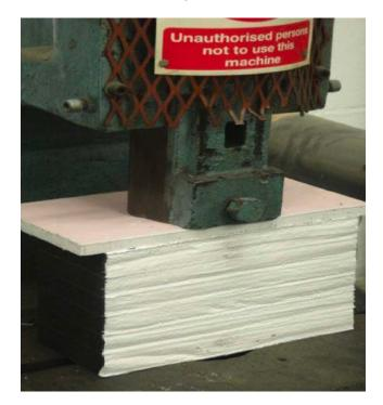
**FlexiCoat-MAK** under 7 tonne load pressure allowing compression to less than 80mm.
