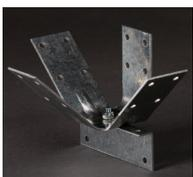
**GRIDLOK® C CHANNEL** - Designed and tested to provide a consistent maximum 280kg/f of bracing capacity to the C Channel rail of plasterboard ceiling systems. Simple click fit and screw off process dramatically reduces time required to complete back bracing. Plenum height chart provide guidance on steel stud BMT required for bracing arms. Features the ability to rotate the unit through 360° minimising service clashes. **STOCK CODE: GRD-10C**
