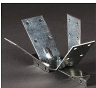
**GRIDLOK® SCREW FIX TCR** - Designed and tested to provide a consistent maximum 280kg/f of bracing capacity to the top cross rail of plasterboard ceiling systems. Simple click fit and screw off process dramatically reduces time required to complete back bracing. Plenum height chart provide guidance on steel stud BMT required for bracing arms. Features the ability to rotate the unit through 360° minimising service clashes. **STOCK CODE: GRD-10S**
