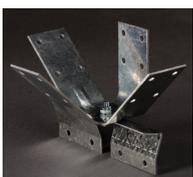
**GRIDLOK® PEAK FORM** - Designed and tested to provide a consistent maximum 280kg/f of bracing capacity to higher profile two-way grid ceiling systems and dry wall grid systems. Simple click fit and screw off process dramatically reduces time required to complete back bracing saving cost to project. Plenum height chart provides guidance on steel stud BMT required for bracing arms. Features the ability to rotate the unit through 360° minimising service clashes. **STOCK CODE: GRD-10P**
